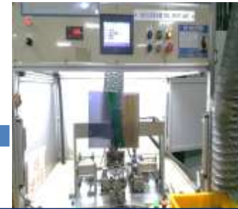
Sub Ass'y + Shaft ( TIG Welding & Torque Test )
